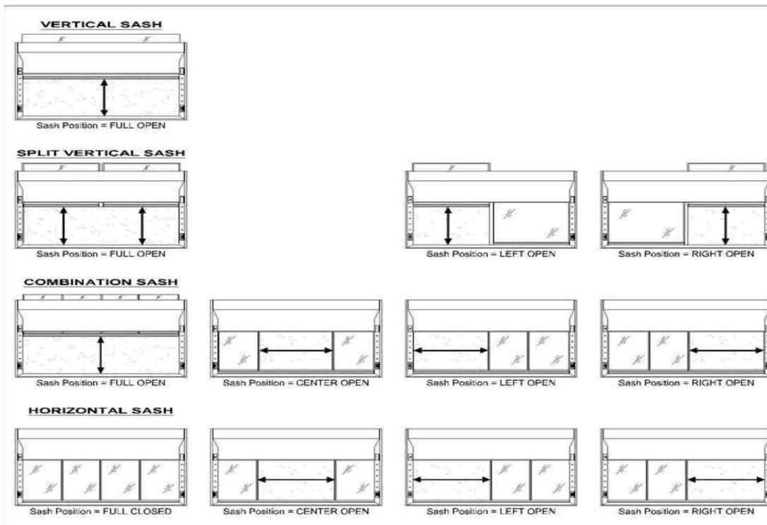
Fig. 4 Typical Sash Configuration for Different Sash Types
