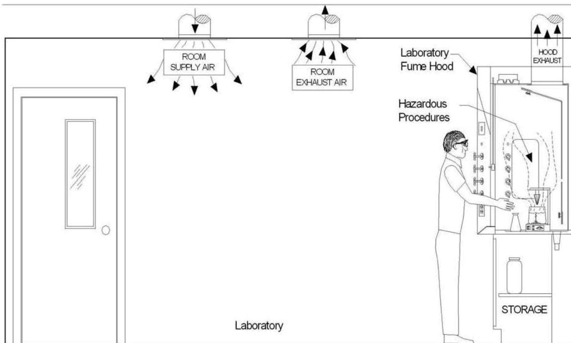
Fig. 1 Typical Constant Volume Laboratory Ventilation System
