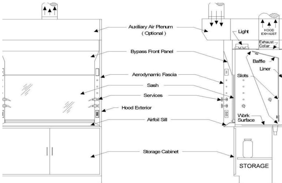
Fig. 3 Typical Components of a Bench Top Hood
