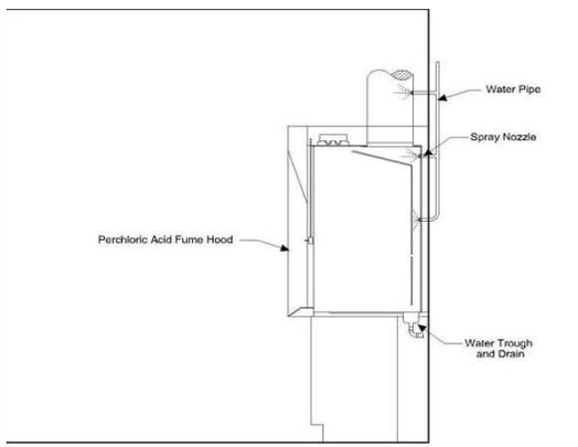
Fig. 6 Typical View of Perchloric Acid Fume Hood
